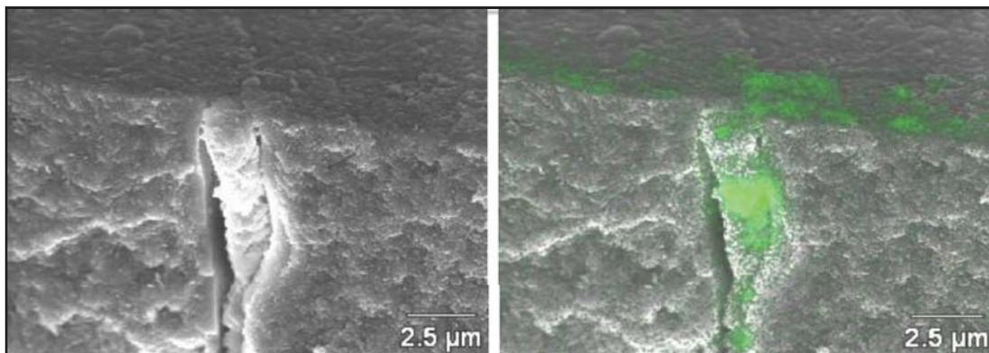
Fig. 6. SEM and EDX elemental mapping of cross-sectioned dentin after treatment with Test Dentifrice 1. The silicon EDX map indicated in green is overlaid on the SEM image (right).
